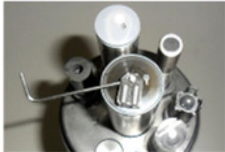
Figure 17: Turbidity Wiper Replacement
