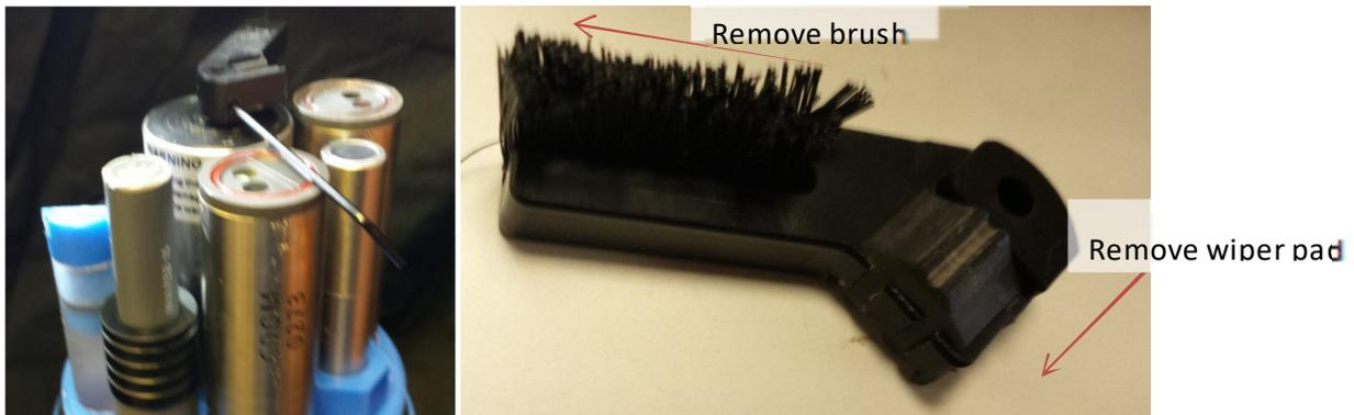
**Figure 21.**(a) Location of set screw for removing the wiper (b) brush arm with wiper pad and brush highlighted
