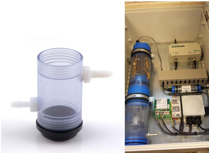
Figure 15: Proteus flow cell with barbed connectors.
