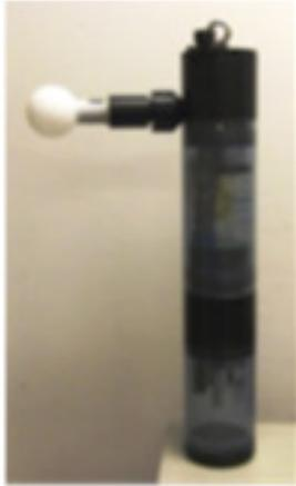
PAR sensors are supplied with a dummy plug so that you can use the Proteus without the PAR sensor attached.
